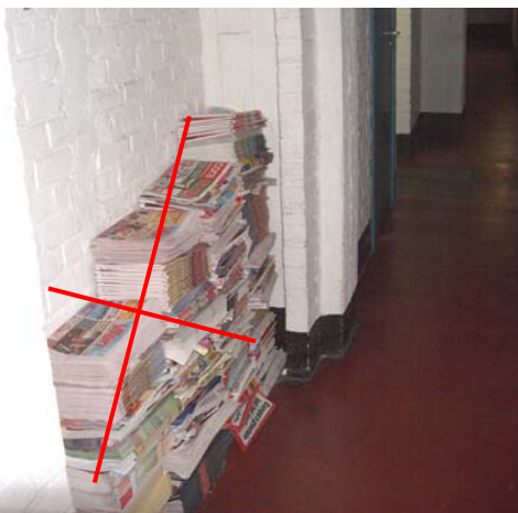
To be avoided! Newspapers lying about in a basement passage, the perfect fuel for any malicious act (source [8])
