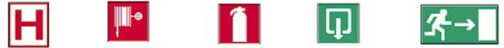
Regulatory pictograms indicating the presence of a hydrant, hose reel, extinguisher or emergency exits
