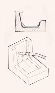
two ~ spray concrete into the mold
