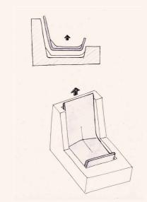
four ~ remove the model from the mold
