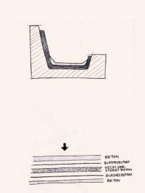
three ~ reinforce with fiberglass layers
