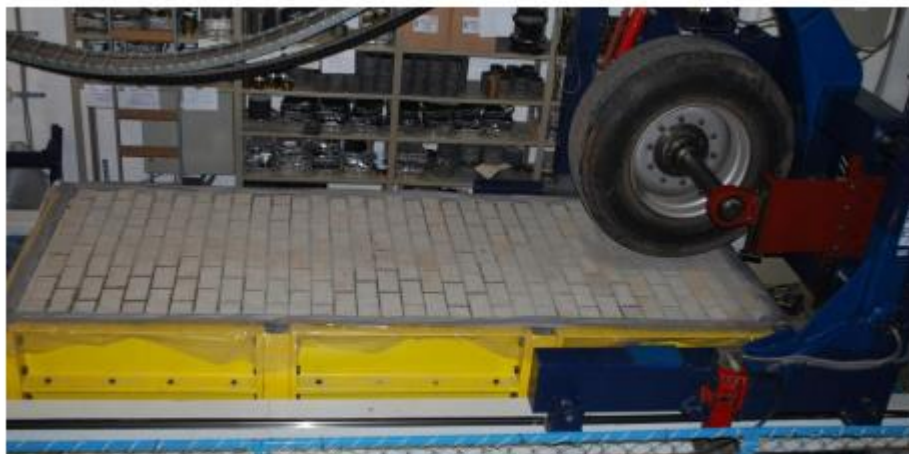
Figure 2. Picture of the RUB-StraP with installed block pavement
