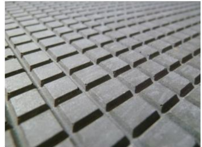
Figure 3. Surface of the produced prefabricated parts in UHPC.
